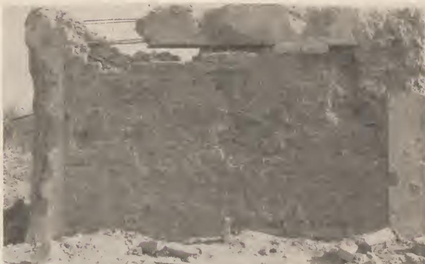
Test B—Panel No. 3 after static detonation of 300-pound demolition bomb at 25 feet.
