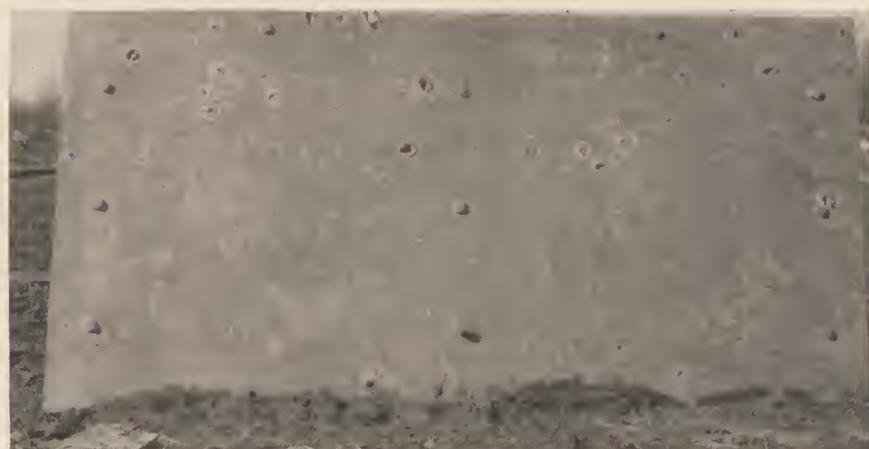
Test B—Panel No. 7 after static detonation of 300-pound demolition bomb at 25 feet.
