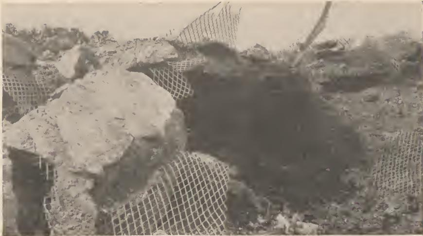
Bomb hits Nos. 36 and 37. Effects of hits on burster slab No. 3 made by 600-pound demolition bombs with delay-action fuses.
