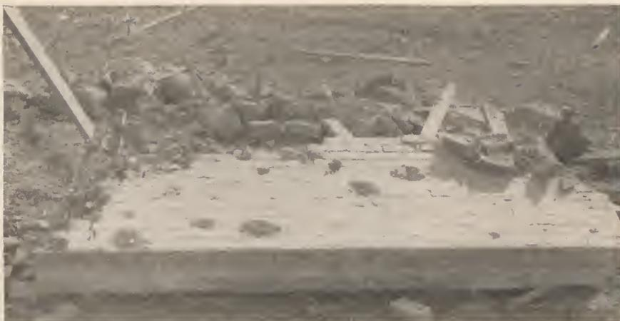
Test B—Panel No. 2 after static detonation of 300-pound demolition bomb at 25 feet.
